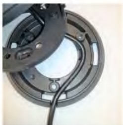
Step 1: Install cable into Wall assembly plate.
